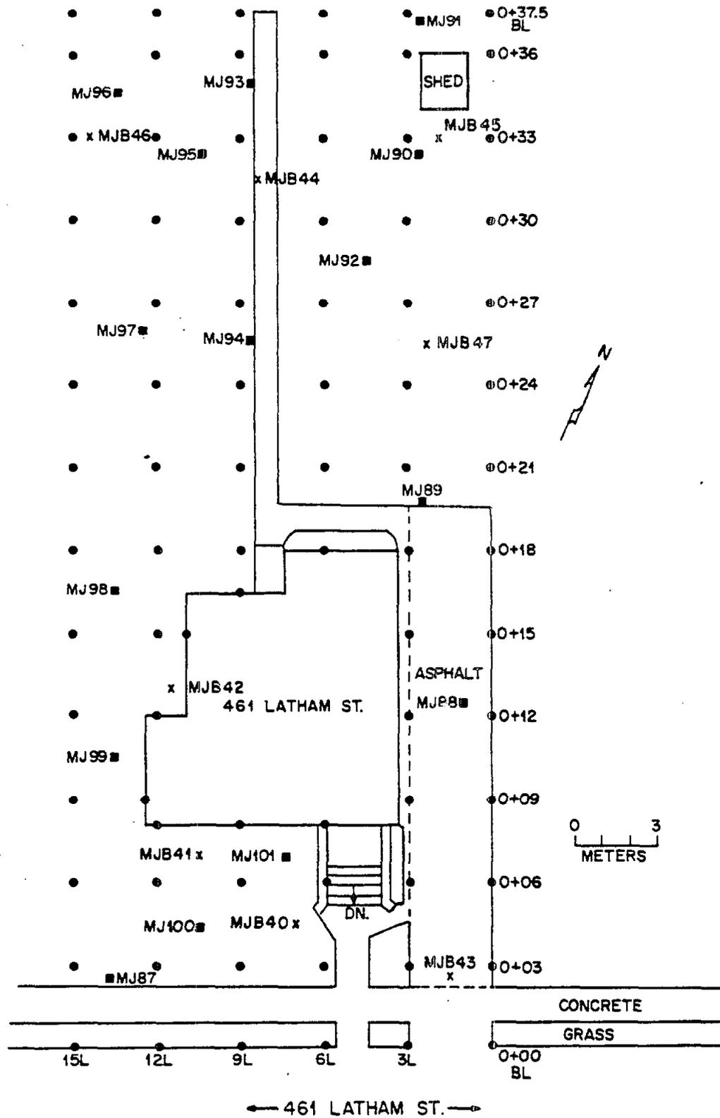
Fig. 5. Location of systematic (MJ) and biased (MJB) soil samples at 461 Latham Street
