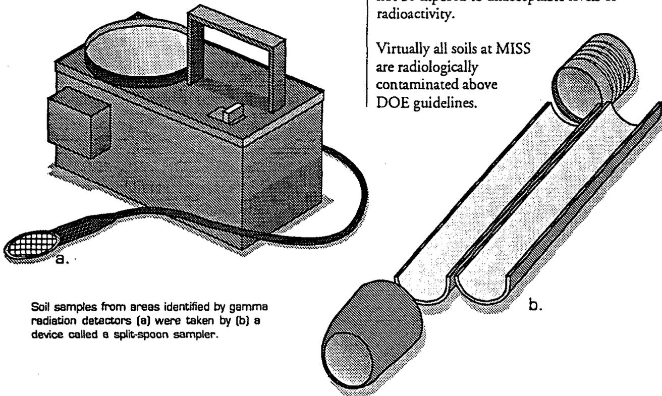
Soil samples from areas identified by gamma radiation detectors (a) were taken by (b) a device called a split-spoon sampler.
