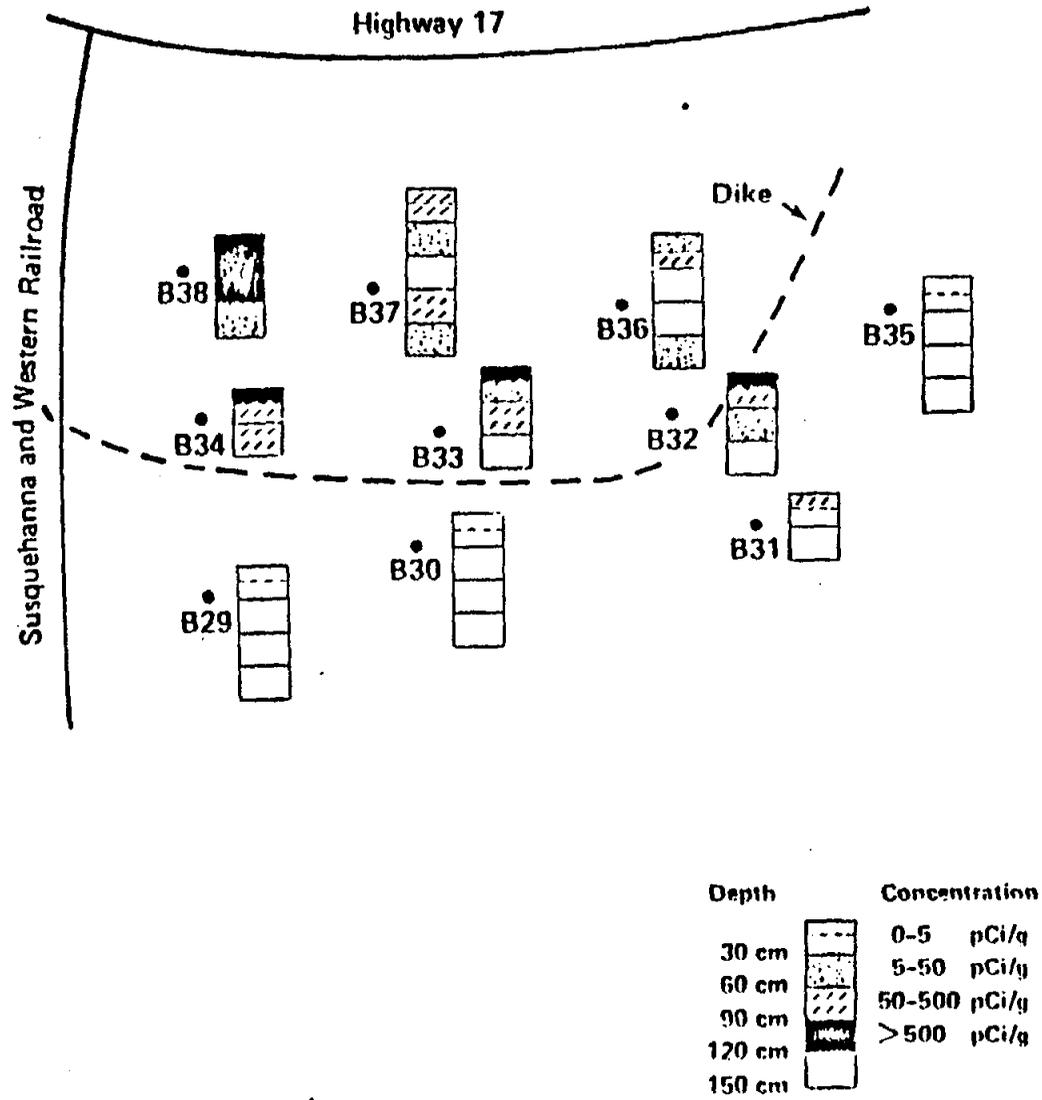
FIGURE 12. View of Northeast Corner of Property With Subsurface Th-232 Concentrations Indicated.
