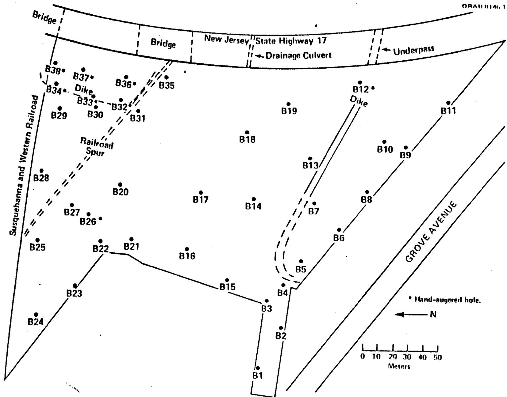
FIGURE 4. Locations of Boreholes and Subsurface Soil Samples.
