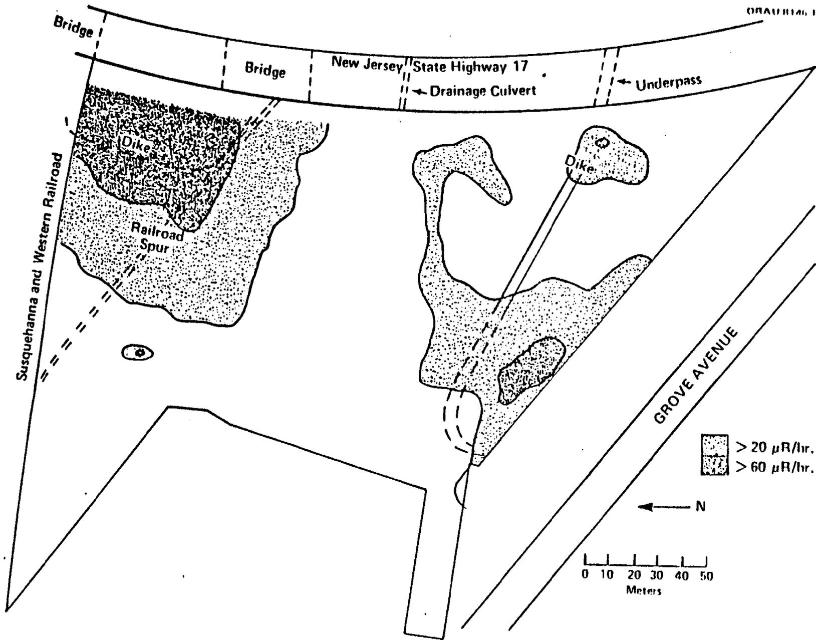
FIGURE 9. Plan View Indicating Gamma Radiation Isopleths at One Meter Above the Surface (background subtracted).
