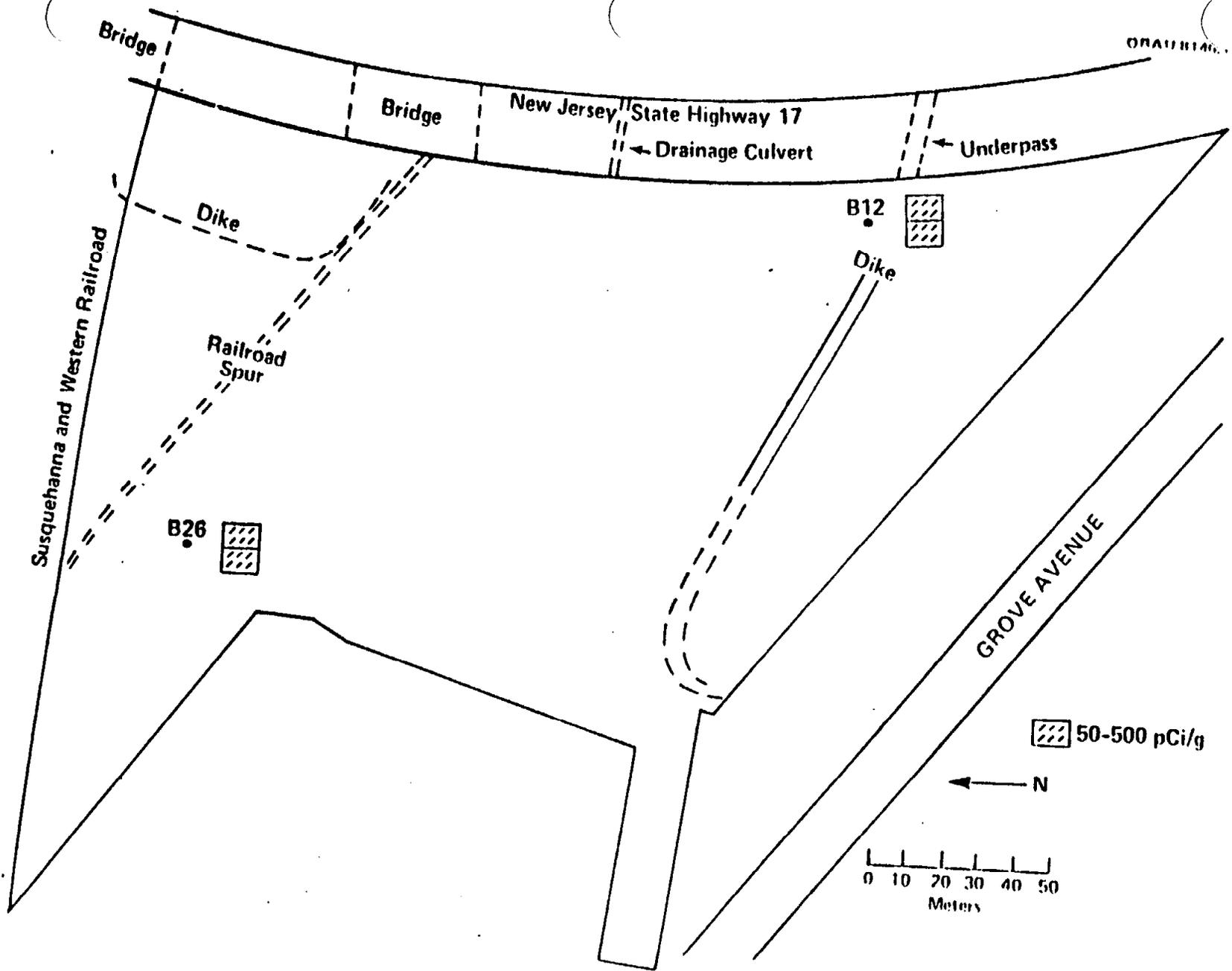
FIGURE 13. Plan View With Subsurface Th-232 Concentrations Indicated for Boreholes B12 and B26.
