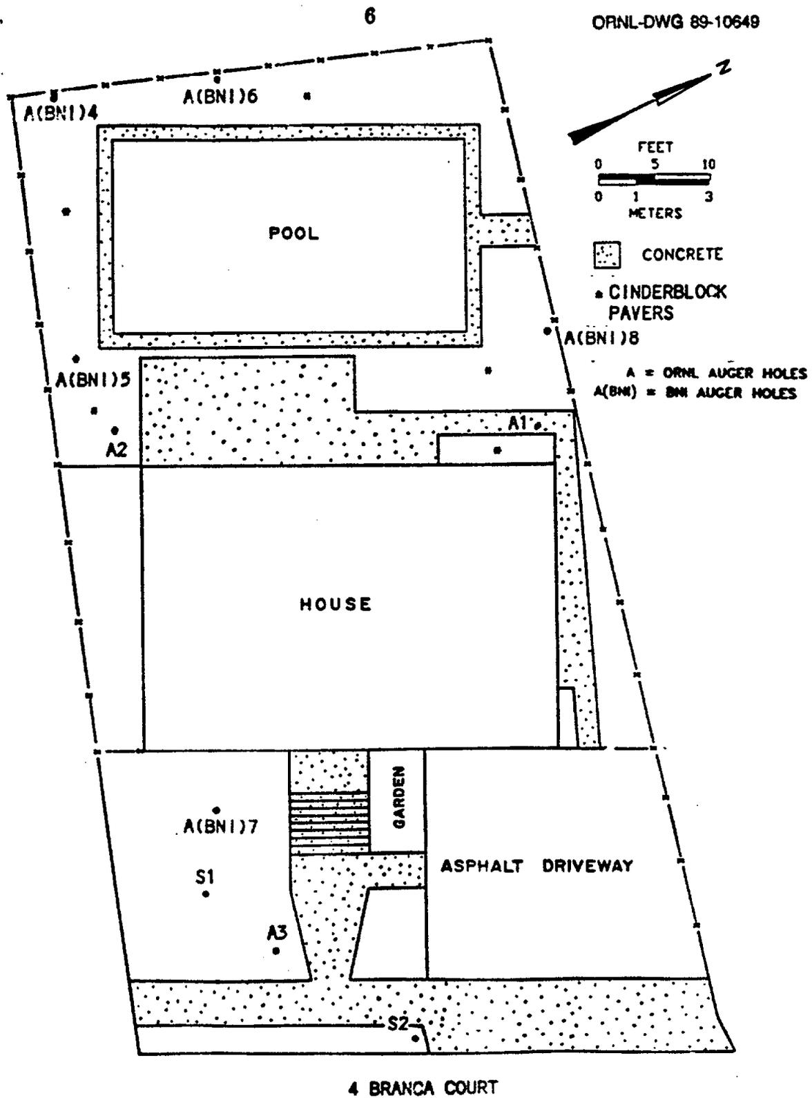
Fig. 2. Diagram showing locations of soil samples taken at 4 Branca Court, Lodi, New Jersey (LJ037).
