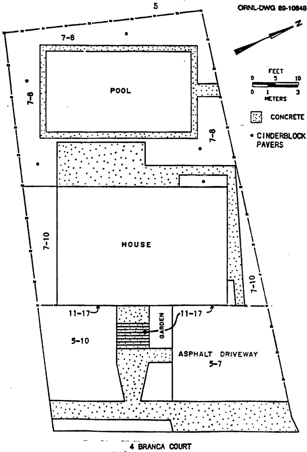
Fig. 1. Gamma radiation levels ( $\mu\text{R}/\text{h}$ ) measured on the surface at 4 Branca Court, Lodi, New Jersey (LJ037).
