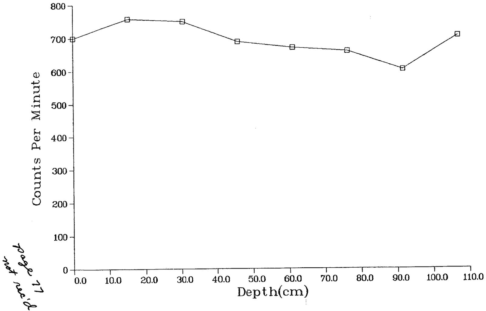
Fig. II-12. Gamma profile of core hole MJC12 (see Fig. 6)
