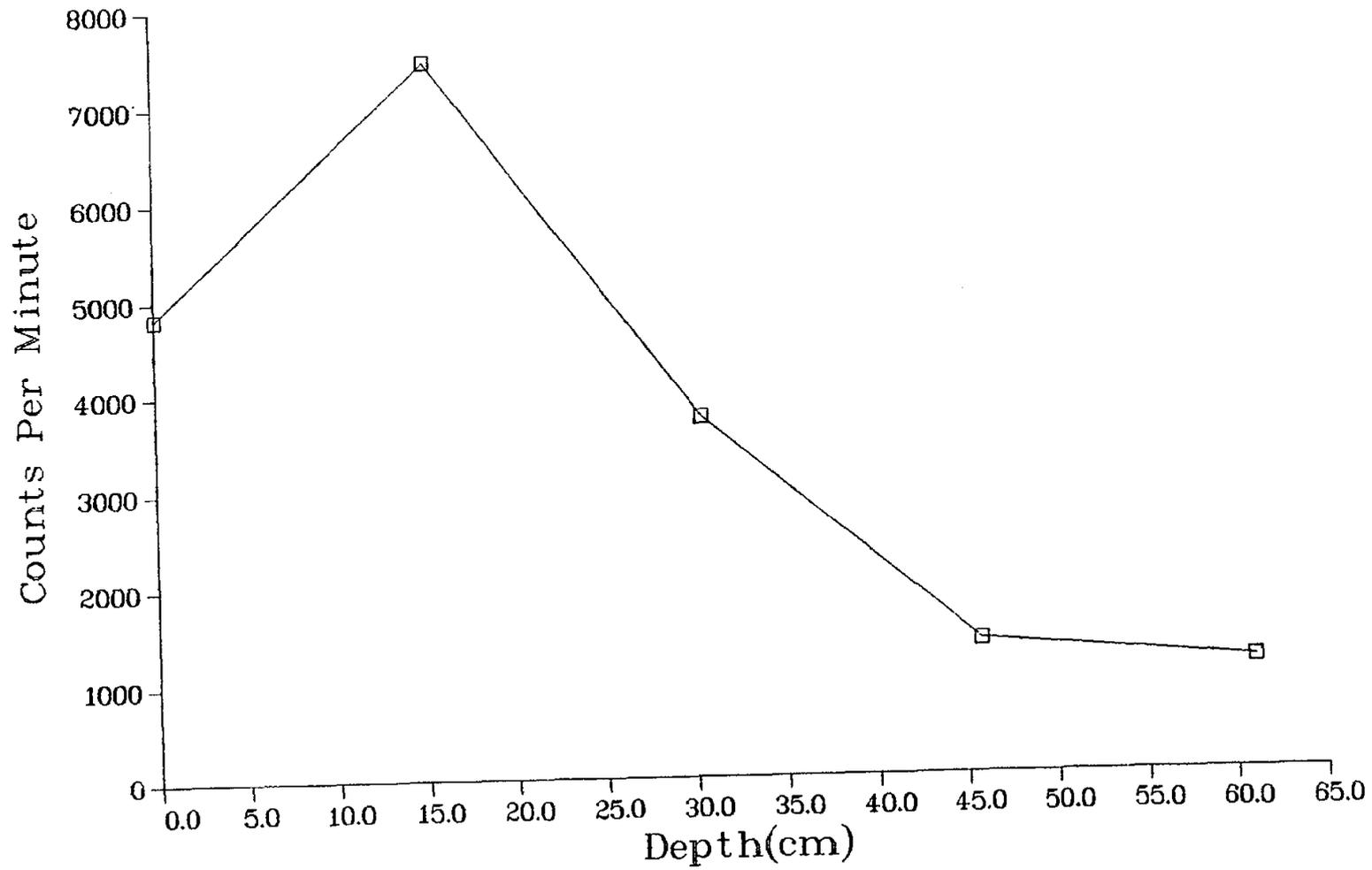
Fig. II-2. Gamma profile of core hole MJC2 (see Fig. 6)
