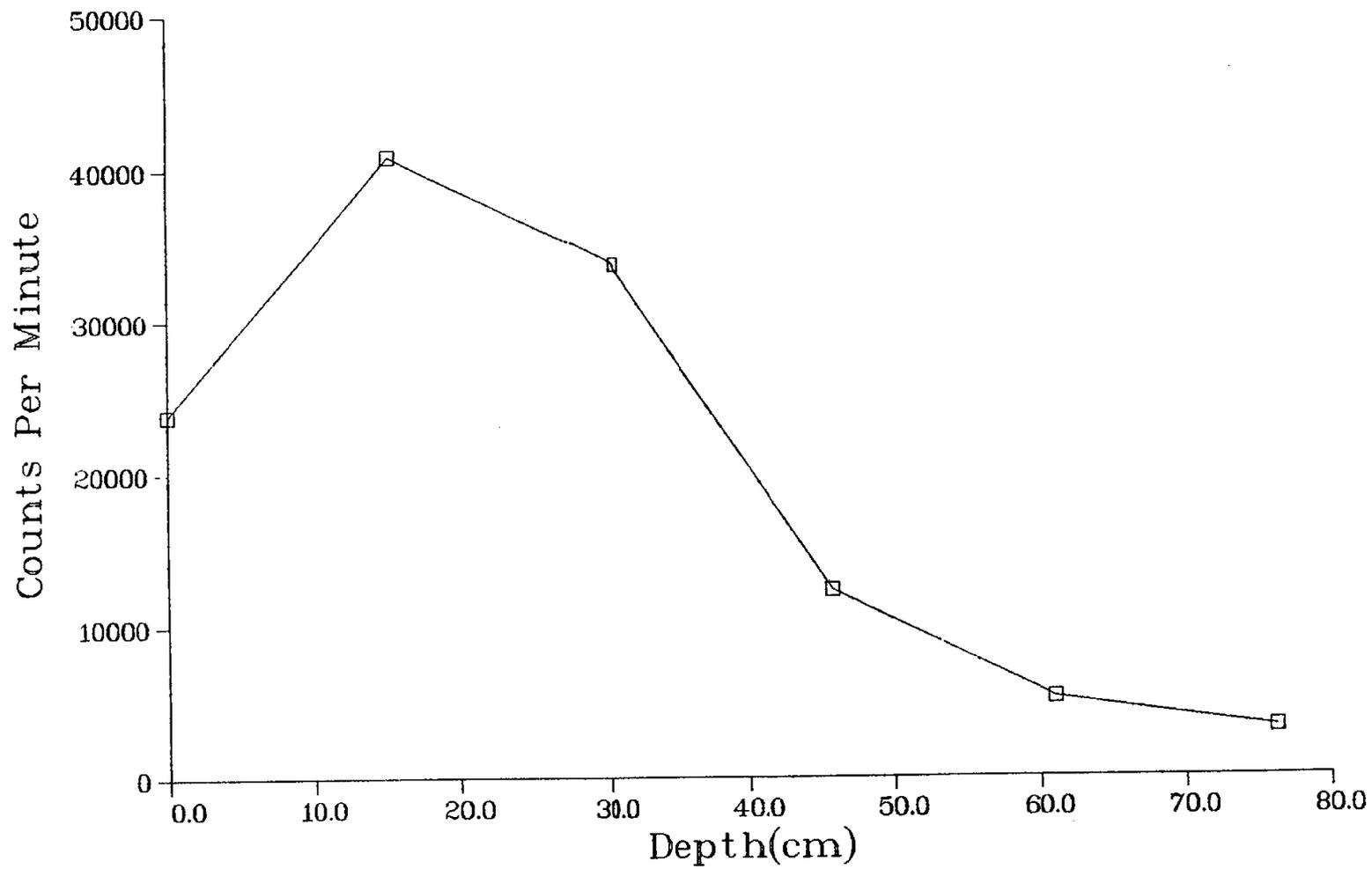
Fig. II-11. Gamma profile of core hole MJC11 (see Fig. 6)
