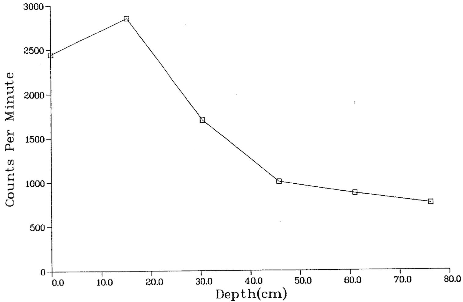
Fig. II-3. Gamma profile of core hole MJC3 (see Fig. 6)
