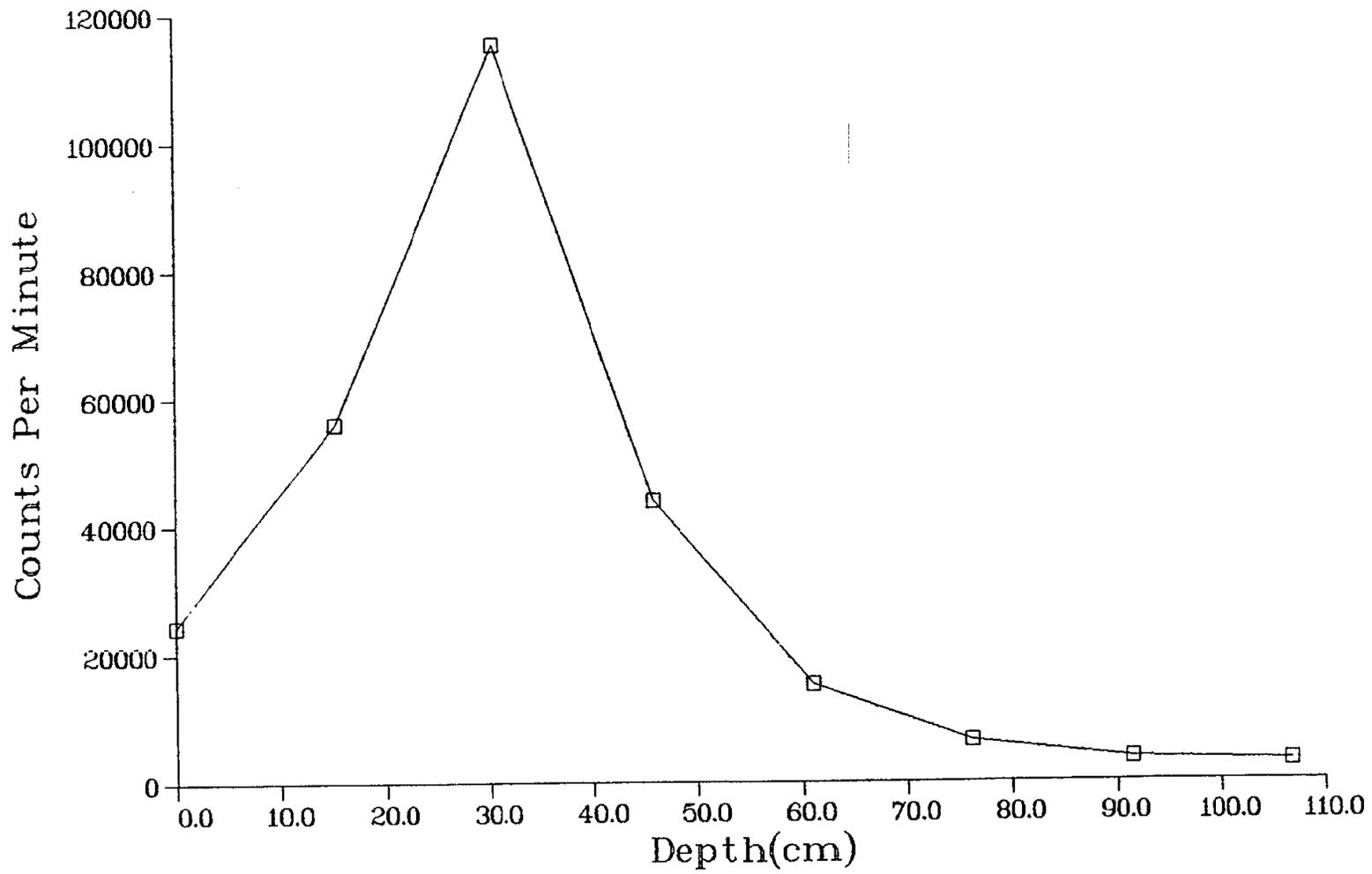
Fig. II-8. Gamma profile of core hole MJC8 (see Fig. 6)
