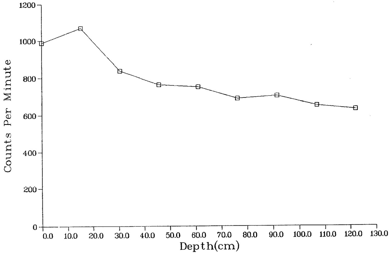
Fig. II-4. Gamma profile of core hole MJC4 (see Fig. 6)
