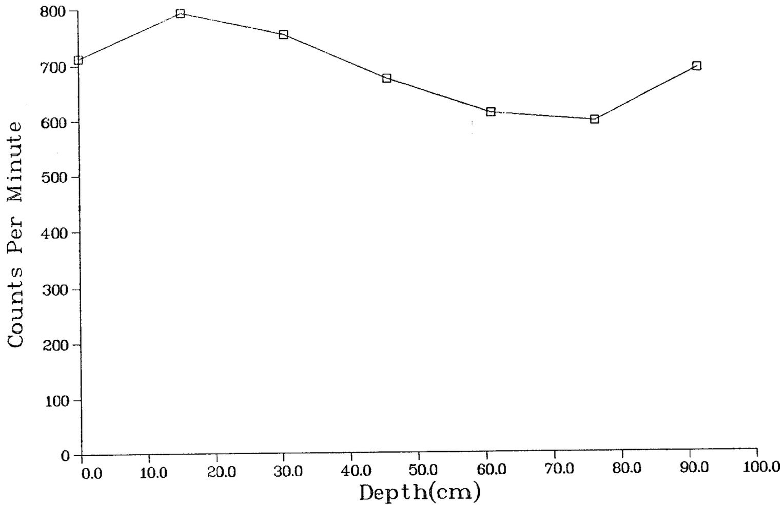
Fig. II-16. Gamma profile of core hole MJC16 (see Fig. 6)
