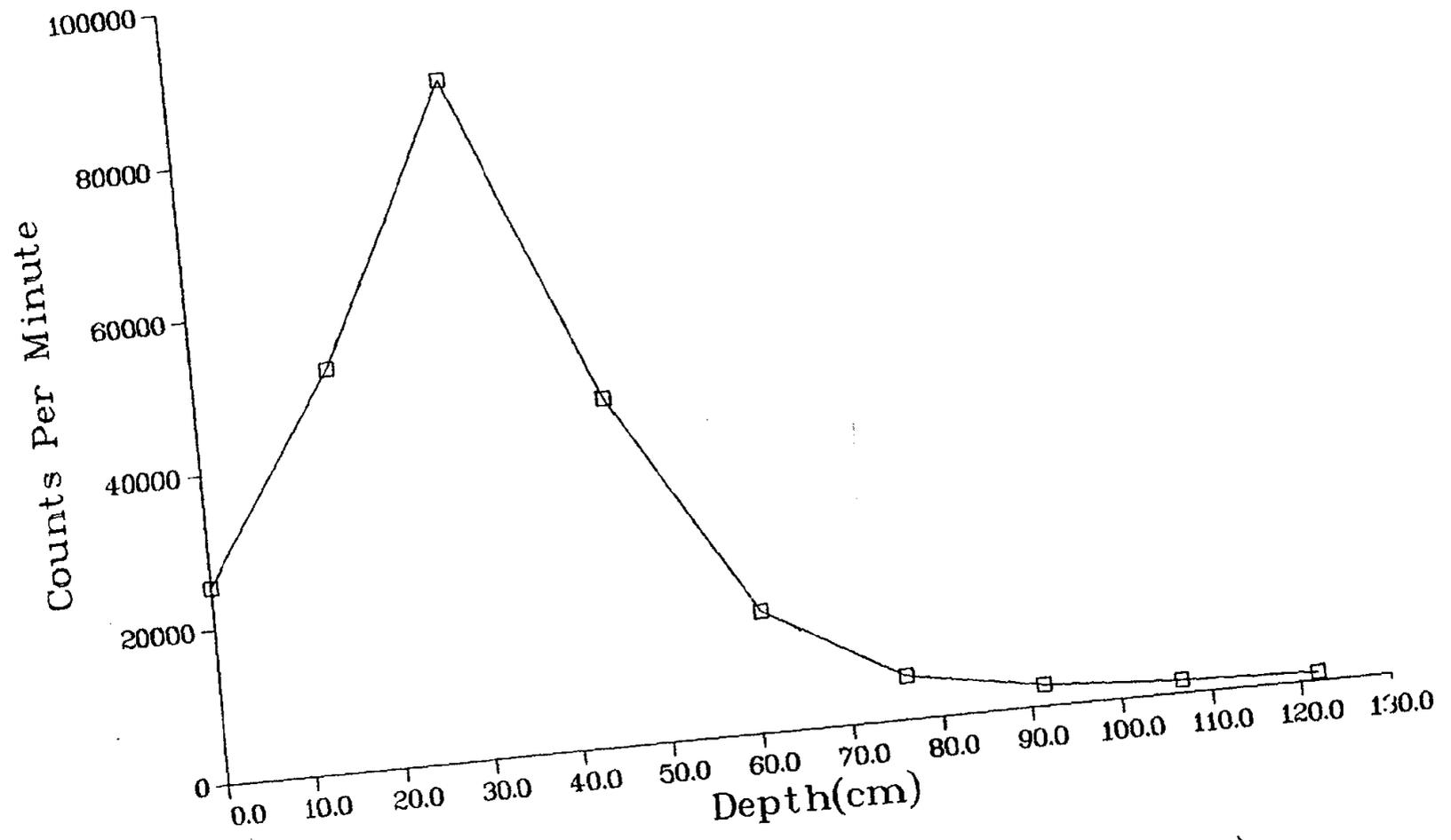
Fig. II-7. Gamma profile of core hole MJC7 (see Fig. 6)
