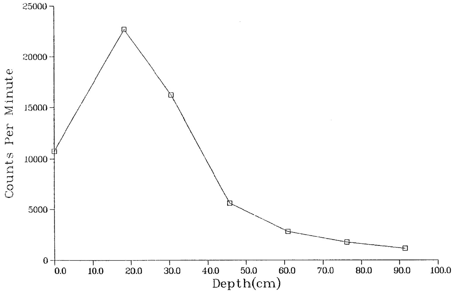
Fig. II-1. Gamma profile of core hole MJC1 (see Fig. 6)
