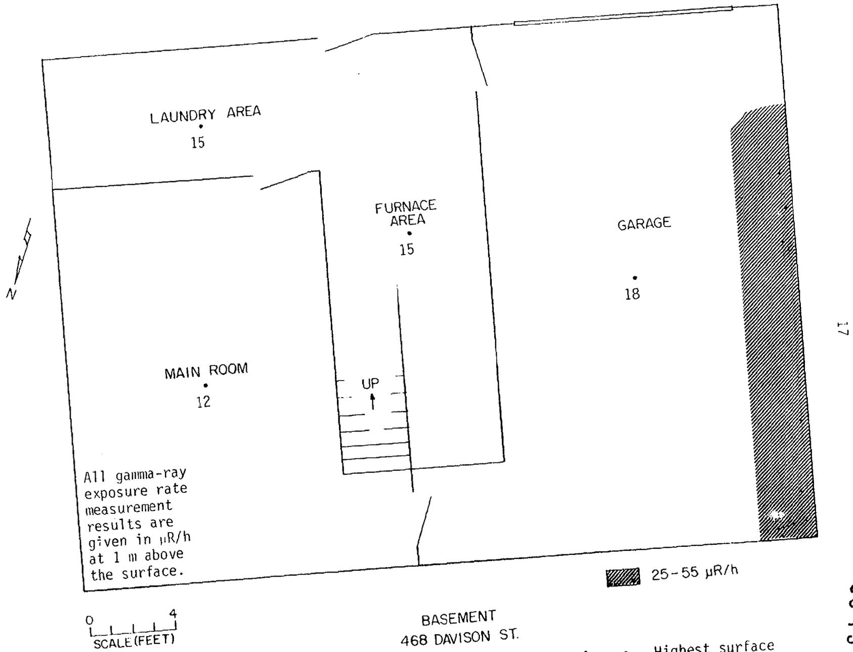
Fig. 9. Schematic of the basement floor plan at 468 Davison Avenue. Highest surface external gamma-ray levels are shaded
