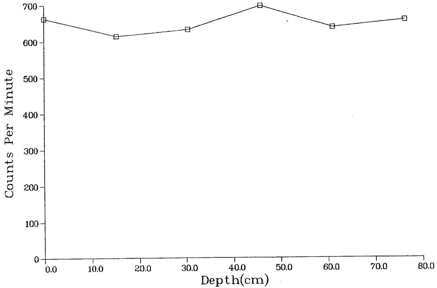
Fig. II-17. Gamma profile of core hole MJC17 (see Fig. 6)
