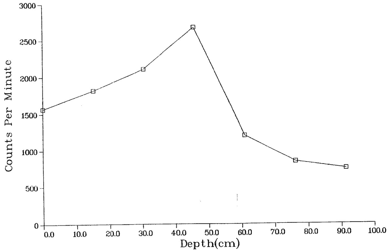
Fig. II-14. Gamma profile of core hole MJC14 (see Fig. 6)
