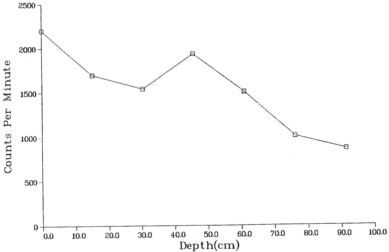
Fig. II-10. Gamma profile of core hole MJC10 (see Fig. 6)
