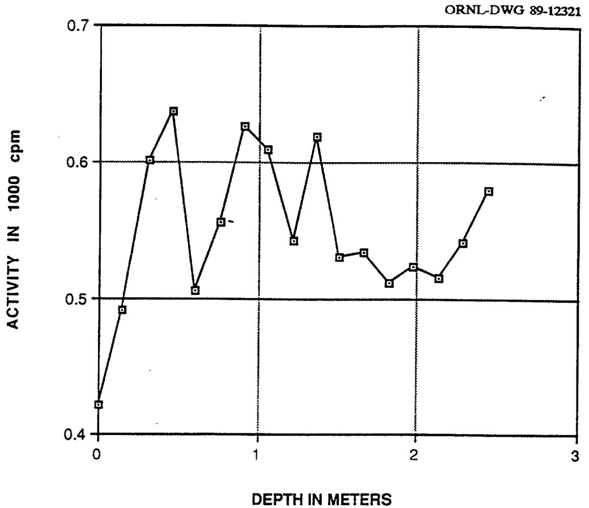
Fig. 7. Gamma profile for auger hole 6 (MJ041A6) at 142 West Central Avenue, Maywood, New Jersey.
