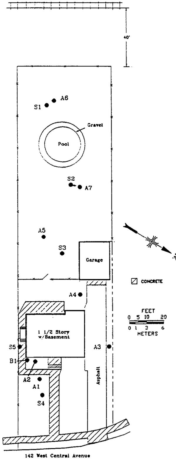
Fig. 2. Diagram showing locations of soil samples taken at 142 West Central Avenue, Maywood, New Jersey (MJ041).
