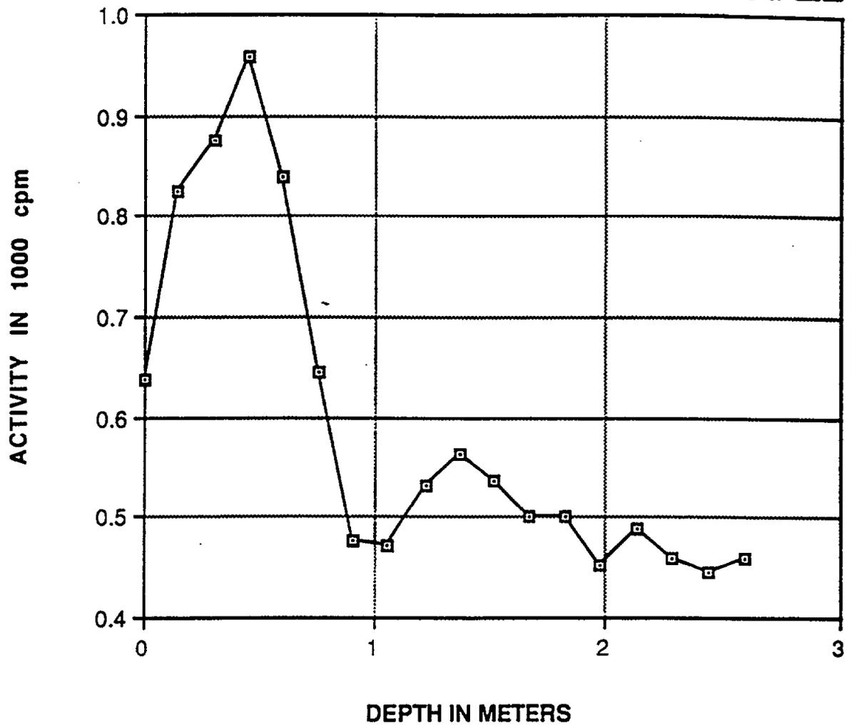
Fig. 8. Gamma profile for auger hole 7 (MJ041A7) at 142 West Central Avenue, Maywood, New Jersey.
